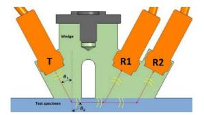
Longitudinal waves can also be used to measure the stresses acting at 90° to the material surface by placing the transmitting and receiving probes directly onto the surface in either a transmission or reflection set-up. By using shear waves however, it is possible to measure the stresses acting parallel to the material surface with a transmission or reflection set-up.
