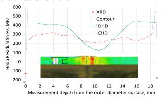
Fig. 2: Hoop residual stress comparison at the WCL
