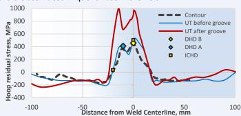
Fig. 7: Ultrasonic measurement across the weld before and after the groove
