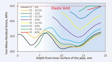
Fig. 5: FE Von Mises residual stresses in the ligament after each increment machined
