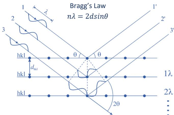
Bi-axial residual stresses are measured using XRD and are nominally accurate to  $\pm 20\text{MPa}$  in steel. The accuracy of the technique is heavily dependent upon good surface preparation and grain size/texture. Although classified as a surface measurement technique, measurements can be made at depths up to 1mm when combined with layer removal.
