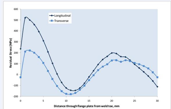
Fig. 4: Residual stresses measured in the full-scale section
