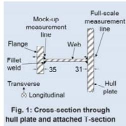
The full-scale component consisted of a circular hull section with dimensions 2360mm long, 6600mm outer diameter and average wall thickness 31mm, see Figure 2. Welded to the inner surface of the hull section were four T-section rings. The final weight of the component was 17 tonnes.
