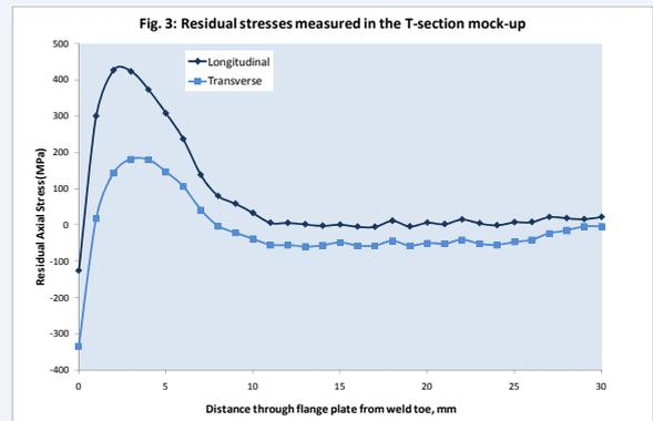
Fig. 3: Residual stresses measured in the T-section mock-up
