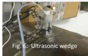
Fig. 6: Ultrasonic wedge
