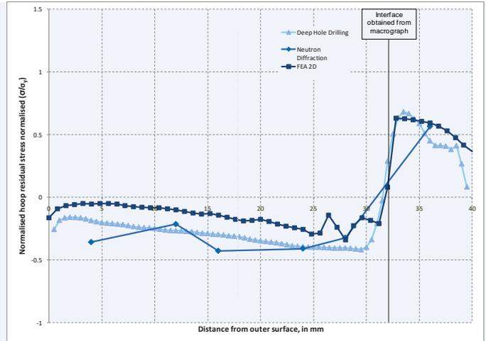
Fig. 3: Comparison of normalised hoop residual stresses measured at 9mm from the weld centreline, i.e. in the ferritic HAZ region.
