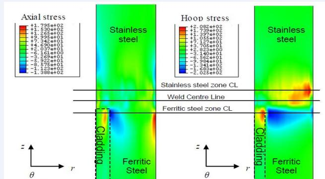
Fig. 5: Estimated residual stresses achieved from measurement mapping
