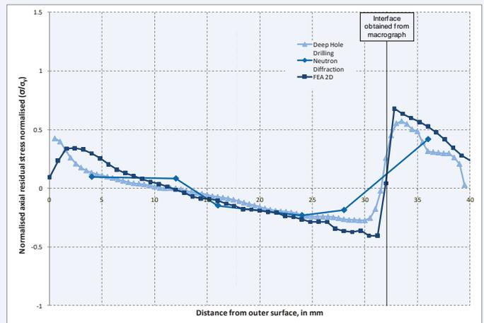
Fig. 4: Comparison of normalised axial residual stresses measured at 9mm from the weld centreline, i.e. in the ferritic HAZ region.
